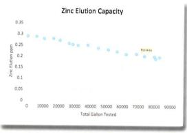
Above graph shows cartridge w/ 30 cubic inches of KDF 55, at 28,500 gallon mark it dropped below the suggested 0.25 ppm spike. However, 0.2ppm Zn for up to 80,000 gallons. Indicating 950g/in^3 is conservative number for bacteriostatic properties to be maintained.
