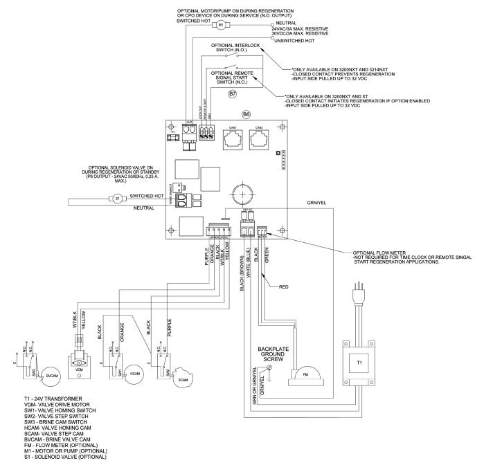
NOTE: 1. TRANSFORMER FUSE - 5A 250V SLOW-BLOW P/N 41143 2. VALVE SHOWN IN SERVICE
